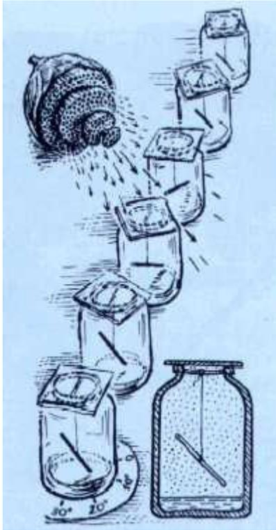
Here they are in the drawing: sealed vessels with straws and burnt twigs-drawing coals-suspended on spider web threads. There is some water at the bottom to counter static electricity hindering experiments in dry air.
